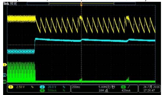
LED Open Fault Happen (CH1-VDD, CH2-VLED, CH4-Primary Current)
