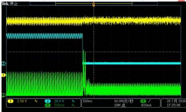
LED Short Fault Happen (CH1-VDD, CH2-VLED, CH4- Inductor Current)
