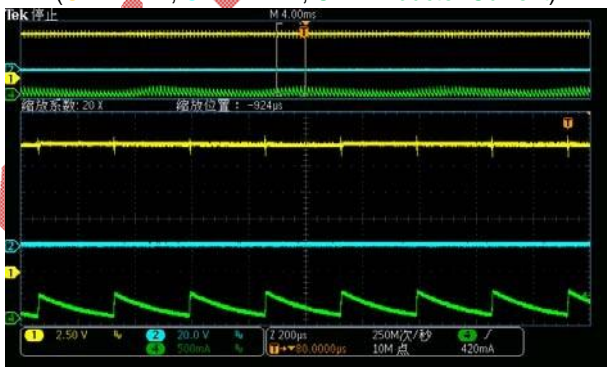
LED Short Fault Steady State (CH1-VDD, CH2-VLED, CH4-Primary Current)
