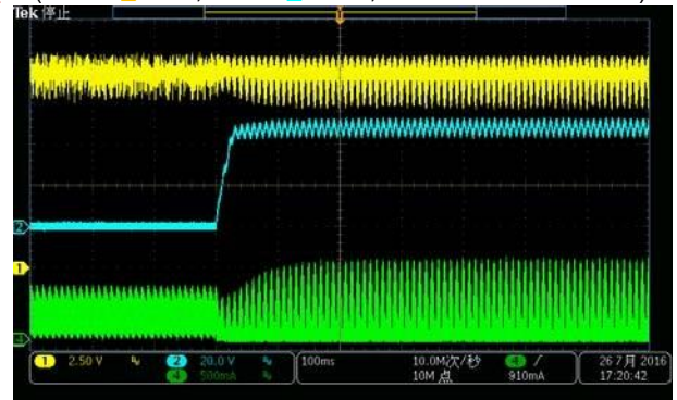
LED Short Fault Recovery (CH1-VDD, CH2-VLED, CH4- Inductor Current)
